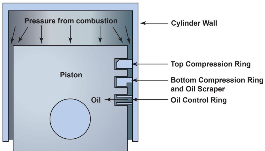
*Combustion pressure forces the compression rings against the cylinder wall to prevent pressure from leaking past the rings and into the crankcase. This would result in a power loss.*
