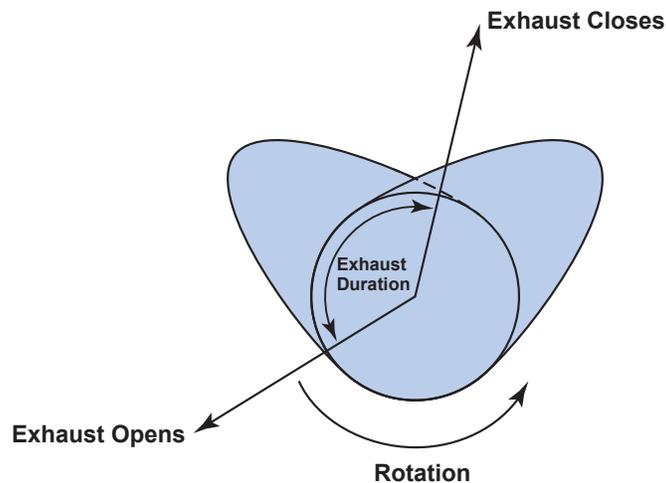
*The profile of the cam lobe determines how long the valve will stay open – referred to as the duration of the cam. This drawing illustrates the exhaust lobe duration.*
