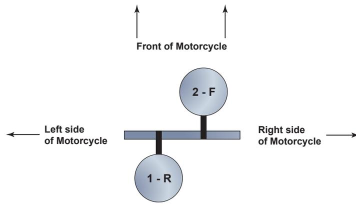
*This V-twin with a transverse crankshaft has the rear cylinder labeled as the number 1 cylinder, and the front cylinder identified as the number two cylinder.*
