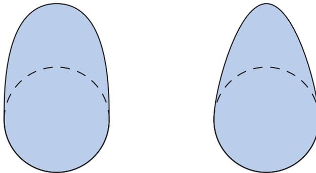
*The cam lobe on the left features a high lift and a long duration. The cam lobe on the right features a high lift and a shorter duration.*
