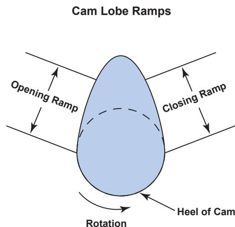
*With the cam lobe rotating counterclockwise, the left side of the cam lobe – the opening ramp – opens the valve. The closing ramp then closes the valve with the help of the valve spring.*
