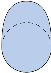
*This drawing illustrates a common cam lobe that is designed for typical motorcycle operating requirements. It features a medium lift and a long duration.*
