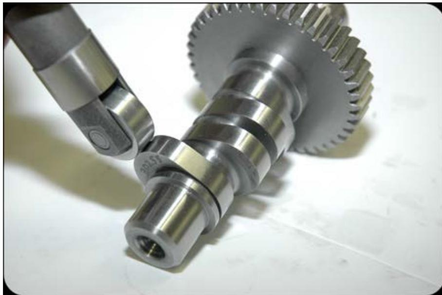
*The cam lobes on this “stock cam” have long duration and a medium lift that is not radical. (Stock Harley evolution camshaft).*
