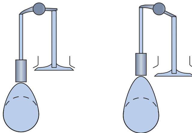
*The high lift cam lobe on the right raises the valve much higher off the valve seat than the lower lift cam lobe on the left.*
