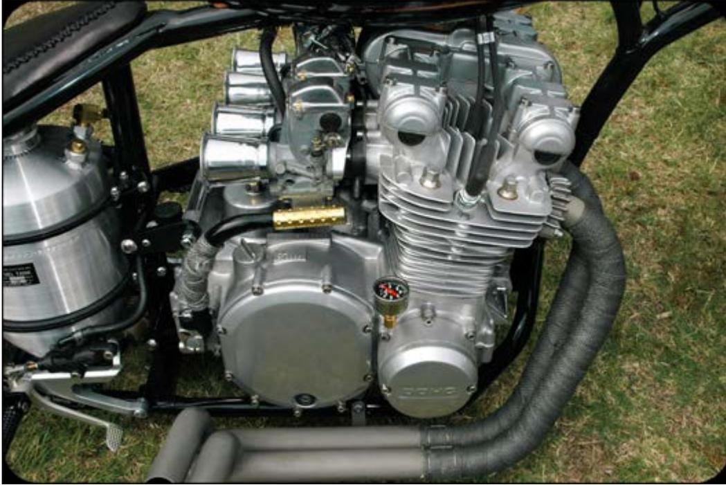
*Photo of an old air-cooled four-cylinder engine where the engine and transmission are housed in one single aluminum case.*
