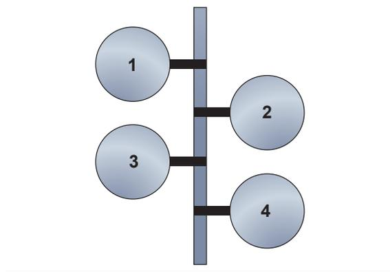
*On a V-4 engine with a longitudinal crankshaft, cylinders may be numbered 1 through 4 from front to back. Note however that numbering can be in a different order depending on the make and model.*
