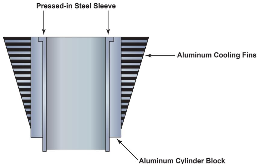
The wall thicknesses of cylinder sleeves are typically in the sizes of 1/16", 3/32" and 1/8". Wall sizes of 3/32" and 1/8" allow for oversize boring later and they are stout enough to preserve the strength of the cylinder block. If sleeves are too thin, the torquing pressure of the head bolts may cause the sleeve to pinch the piston, which causes horsepower losses and high wear from friction.
