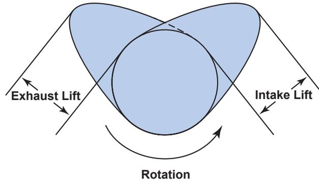
*This illustration displays cam lift. The cam lift and duration changes how and where the engine makes torque and horsepower in the engine power band.*
