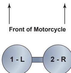
*A parallel twin with transverse crankshaft has a number 1 or “left” cylinder identifier, as well as a number 2, or “right” cylinder identifier.*
