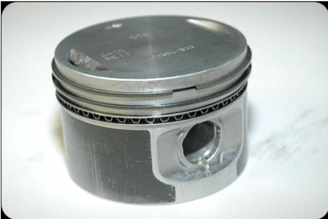
*Side view of piston and three rings. Note the bottom oil scraper that consists of an expander and two flat rings located on either side of the expander. (See prior page)*
