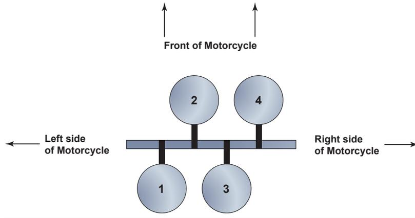
*On a V-4 engine with a transverse crankshaft, cylinders may be numbered 1 through 4 from left to right. A V-4 may receive additional “front” or “rear” identifiers in a service manual, because there are front and rear cylinders.*
