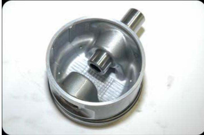
*Bottom of piston shows where piston pin fits through the piston and the connecting rod.*
