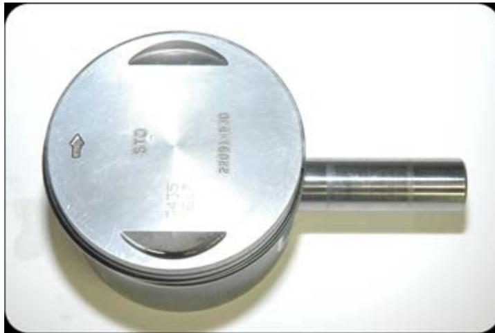
*Flat top piston with cutaways to prevent contact between valves and piston. Arrow must point to the front of the engine to fit piston in correct position due to off-center crankpin. (HD Evolution engine piston).*
