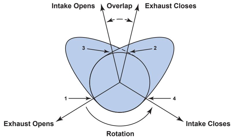
*This somewhat advanced camshaft illustration can be confusing. This common layout has been simplified with numbers that represent certain points. Overlap happens when the exhaust valve is still open for just a short moment while the intake valve is just opening.*
