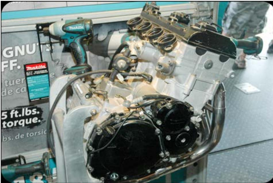
The engine and transmission of this inline four-cylinder engine is contained in a single aluminum engine case.
