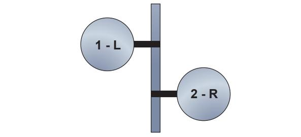
*A V-twin engine with a longitudinal crankshaft has the cylinders labeled as number 1 (left side of crankshaft), and number 2 (right side of crankshaft).*
