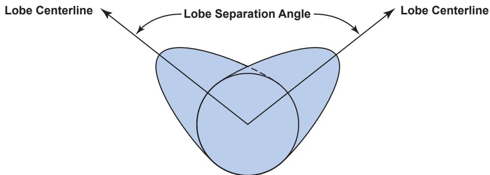
*Cam lobe separation angle is the distance measured in degrees between the centerline of the intake lobe and the centerline of the exhaust lobe. The lobe separation angle determines valve timing and the period of valve overlap. It directly effects how the cam will make power during engine operation.*
