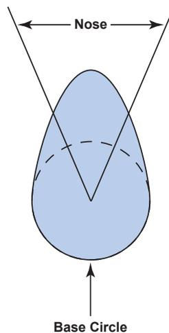
*The base circle is the round “cylinder” part of the cam construction.*
