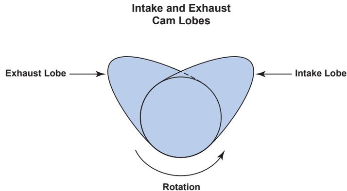
*This illustration displays the intake and exhaust cam lobe and their relationship to each other. In a counterclockwise camshaft rotation, the exhaust valve opens and closes **first** during the exhaust cycle of the engine. After the exhaust valve closes, the intake valve then opens to supply air-fuel mix. Note that the cam lobes are not opposite of each other. The intake lobe performs its job immediately after the exhaust lobe performs its function.*
