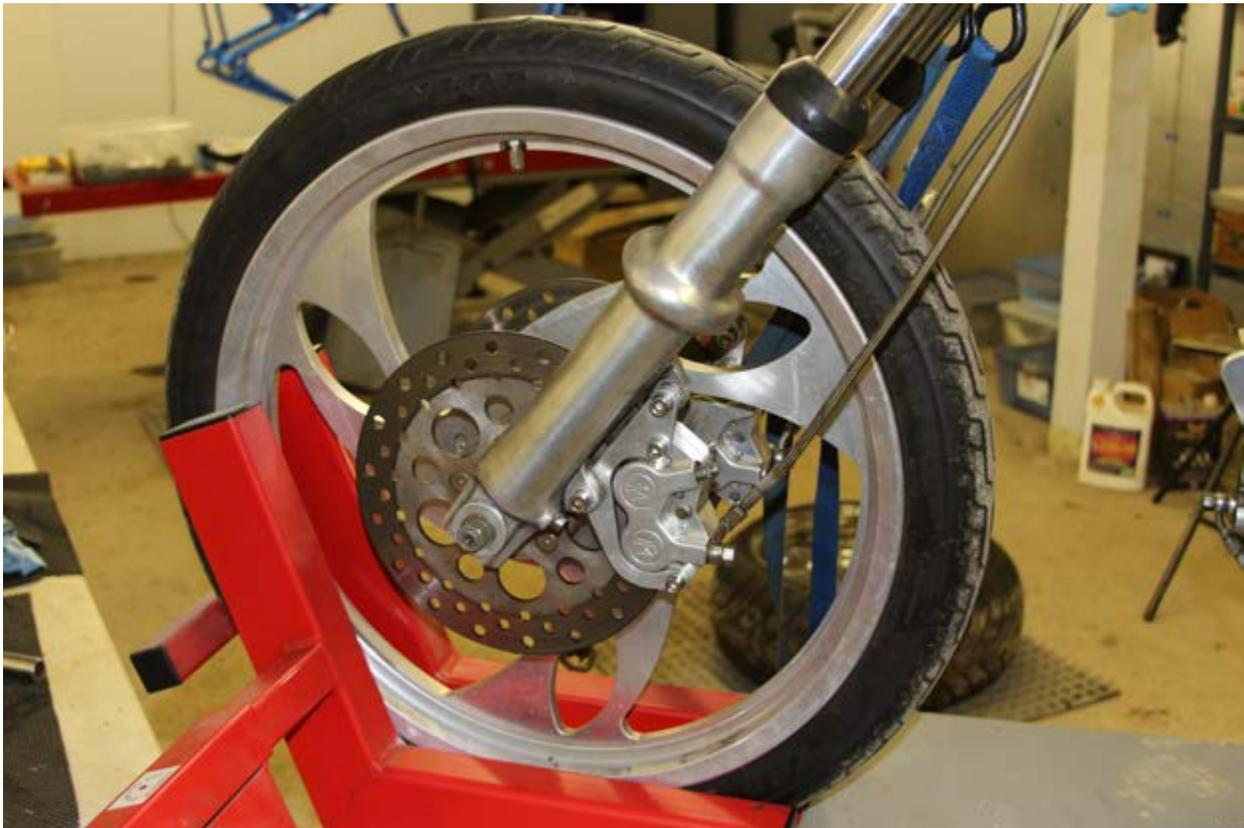
*CNC machines can be programmed to produce billet aluminum wheels with exotic designs.*
