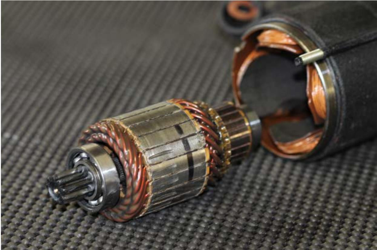
*Starter armature pulled out of the starter case. The commutator is located on the far end of the armature (right side). Brushes inside the end cap ride over the commutator and feed battery current into the armature.*
