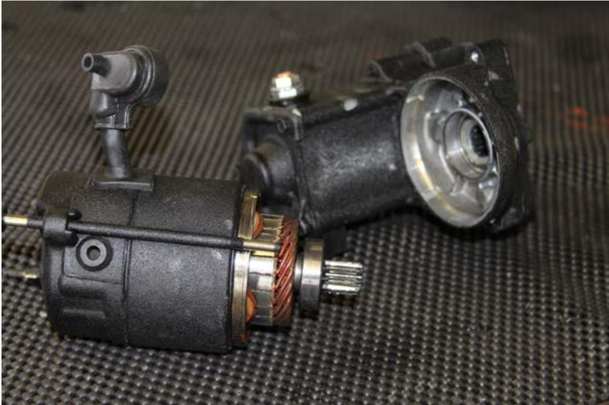
*Starter housing is separated. Starter armature sits between the field coils. The gear on the end of the armature will engage the drive assembly/overrunning clutch gears. The solenoid and housing – top right – has been detached from the starter housing and armature.*
