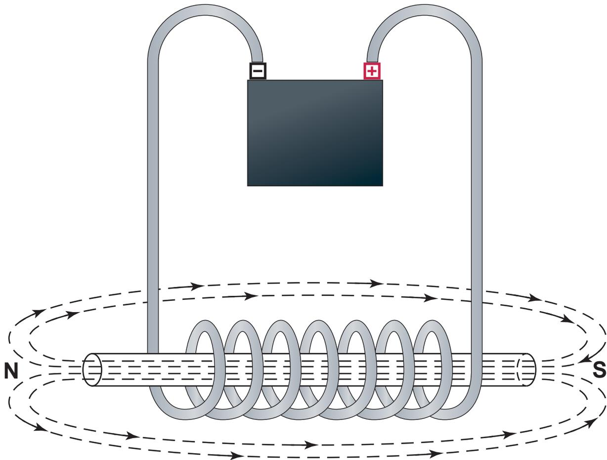
*An electromagnet is created by wrapping a coil of copper wire around a soft iron core and then running electrical current through the wire. This creates a powerful magnetic field in the iron core.*
