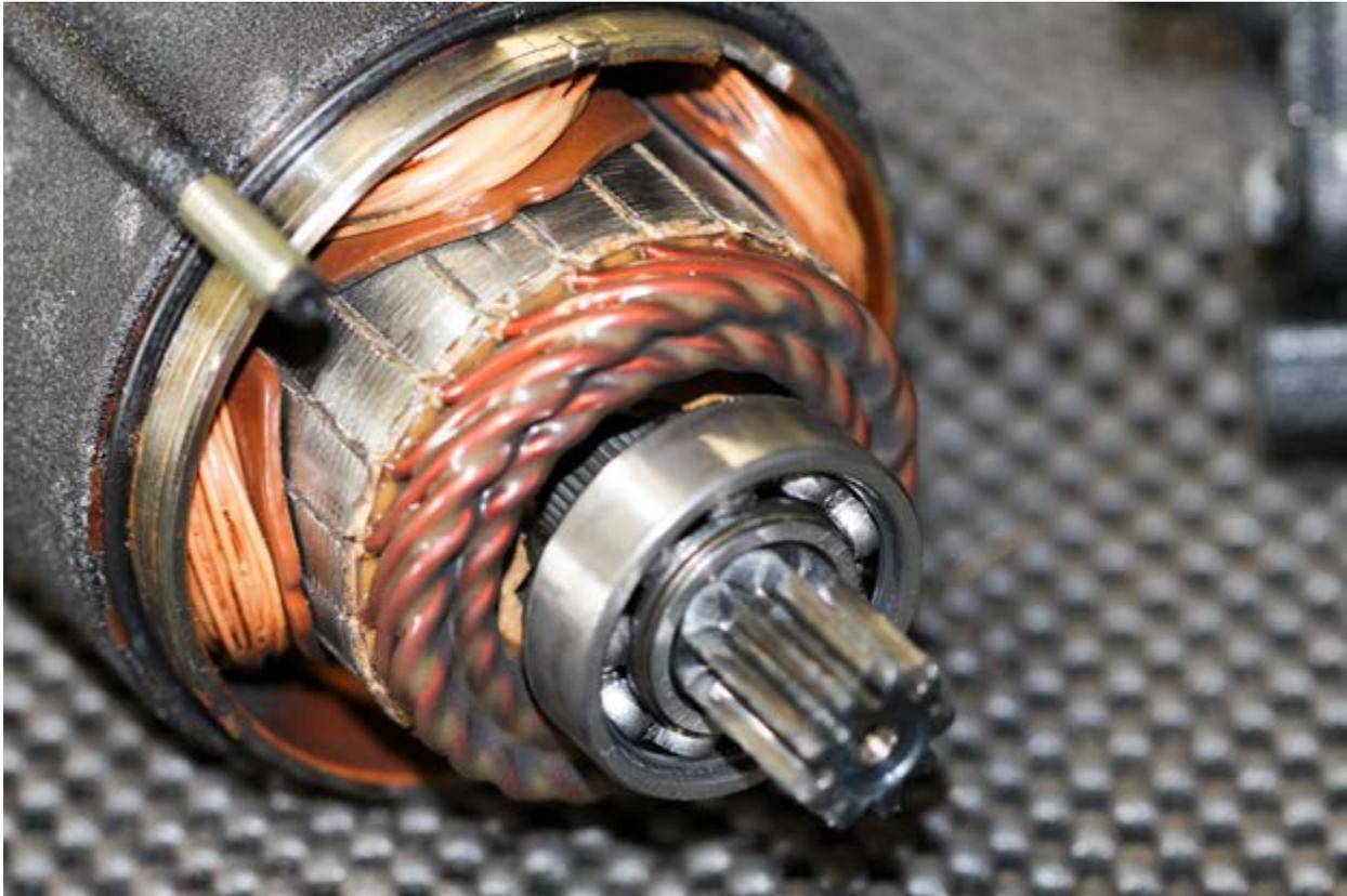
*With starter partially disassembled, notice how the starter armature sits between the field coils. Field coils can be seen on the left and right side, as well as on top. On the end is the gear that will mesh with the starter clutch assembly, and the final starter shaft.*
