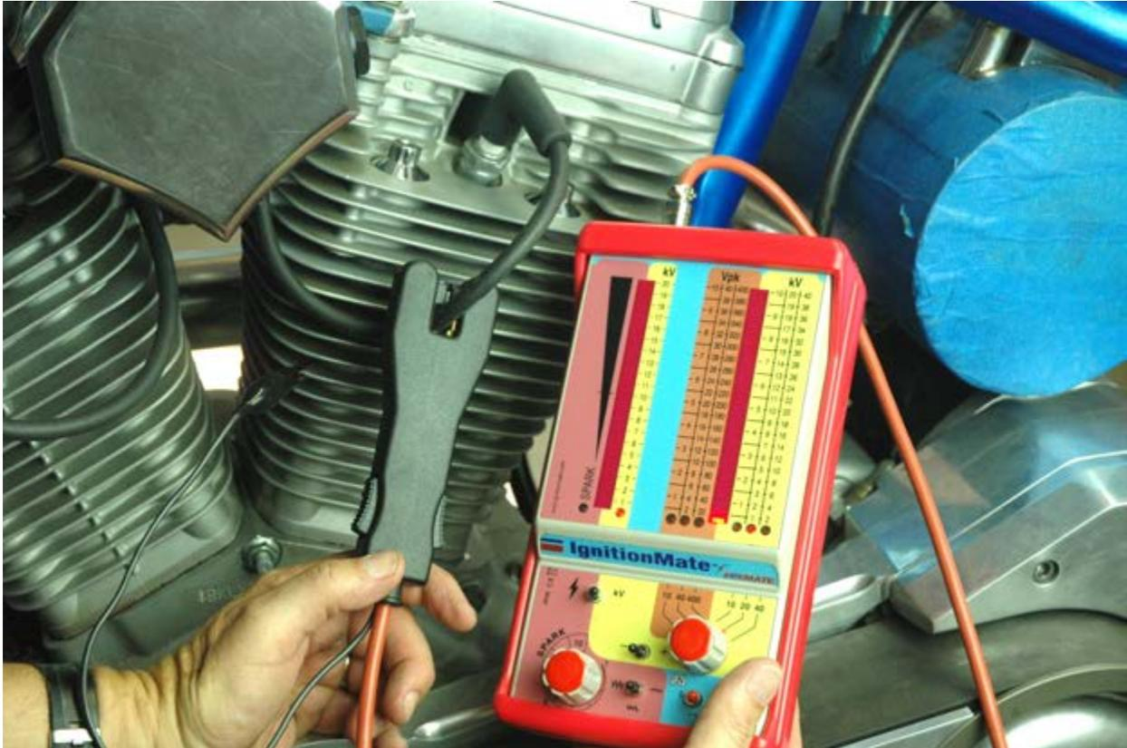
*The IgnitionMate measures the number of volts produced by the secondary circuit of the ignition coil. It can measure up to 40,000 volts. This test quantifies the performance of the ignition system as a whole, based on the strength of the secondary voltage to the spark plug.*
