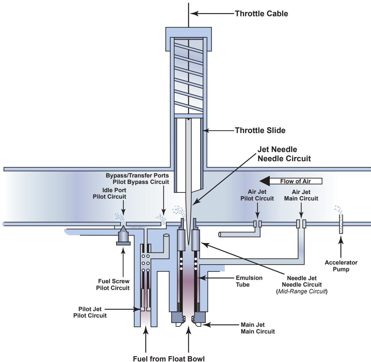
After the air and fuel are mixed together in the mixing chamber, this air-fuel mix then flows through a final passage on its way to the idle discharge hole in the carburetor bore. However, protruding into this final passage is a fuel screw.
