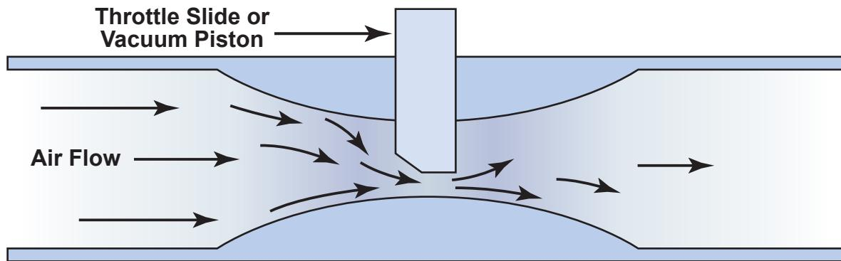
When the throttle slide is raised to allow more air through the bore, the needle attached to the bottom of the slide is also raised at the same time to allow more fuel to flow through the main jet.
