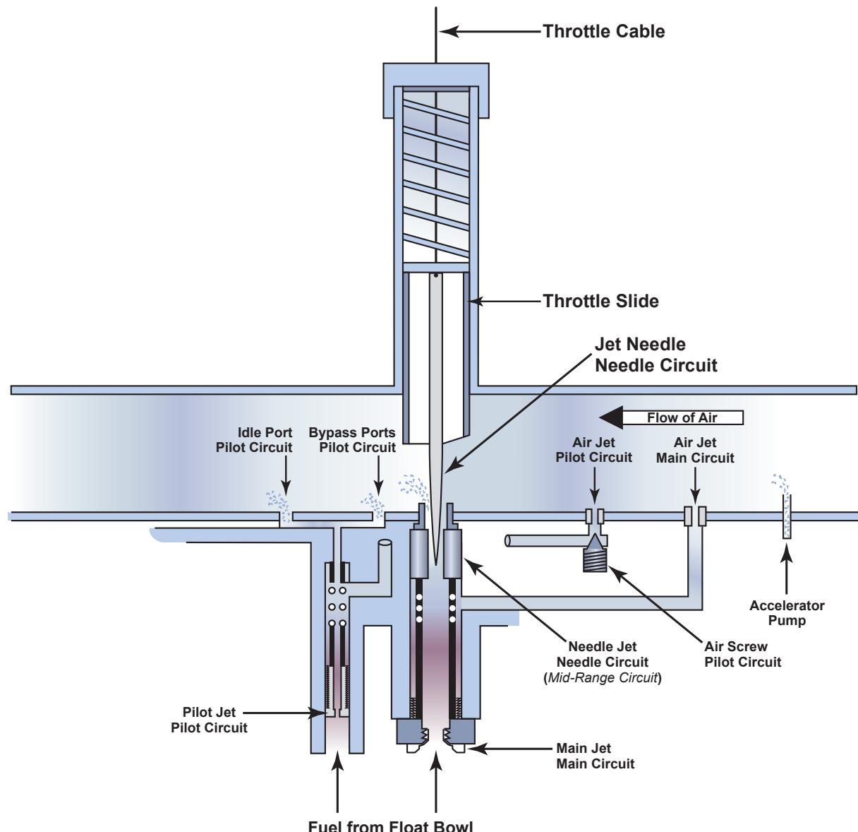
The pilot circuit that is metered with an air screw works as follows:
