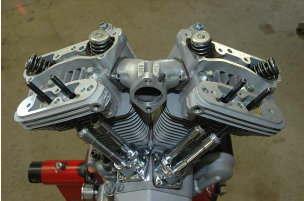
*Cylinder and cylinder head cooling fins on this Harley engine provide the only cooling for the engine in addition to the engine oil.*
