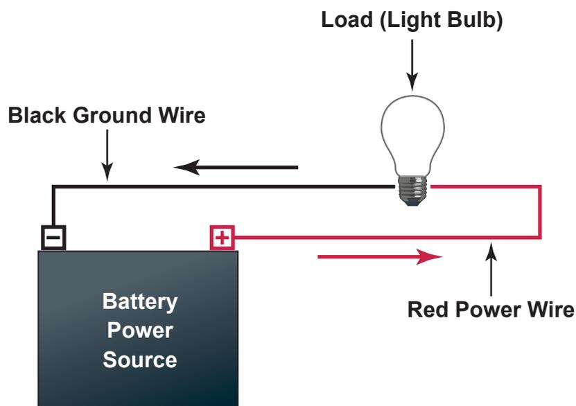
*A basic electrical circuit contains a power source, a conductor to transport the power, a load, and a ground return. The power source here is the battery positive terminal. The red wire is the conductor that transports power to the load. The light bulb is the load. The ground return completes the circuit by returning to the negative battery terminal through the ground wire (conductor).*
