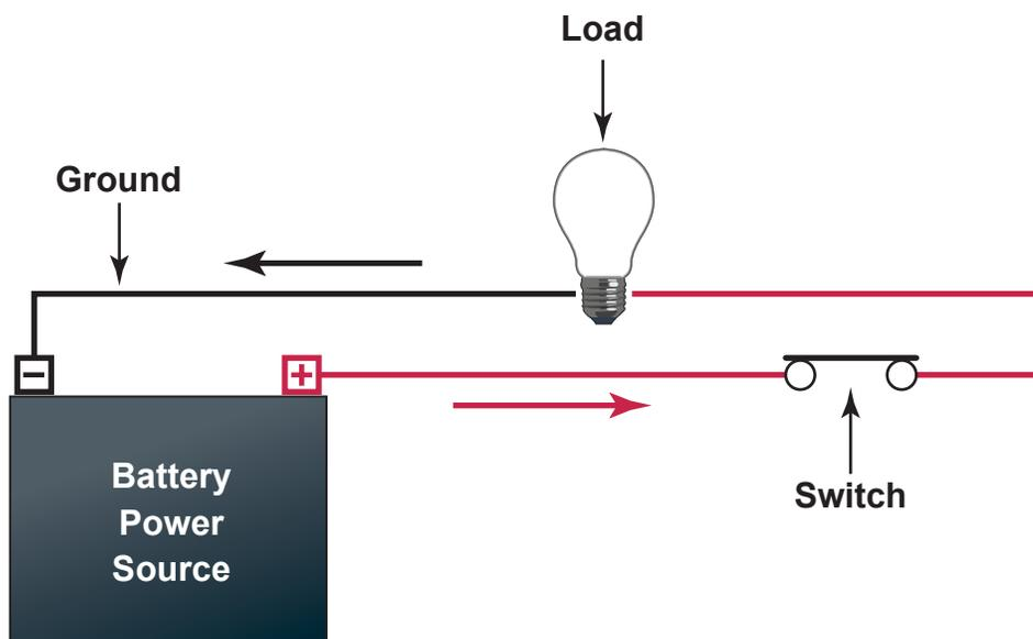
*This basic electrical circuit includes a switch that controls the power to the load. The switch is in the closed position and the circuit is “on” and supplying power to the load. This is a “closed circuit” and it is live.*
