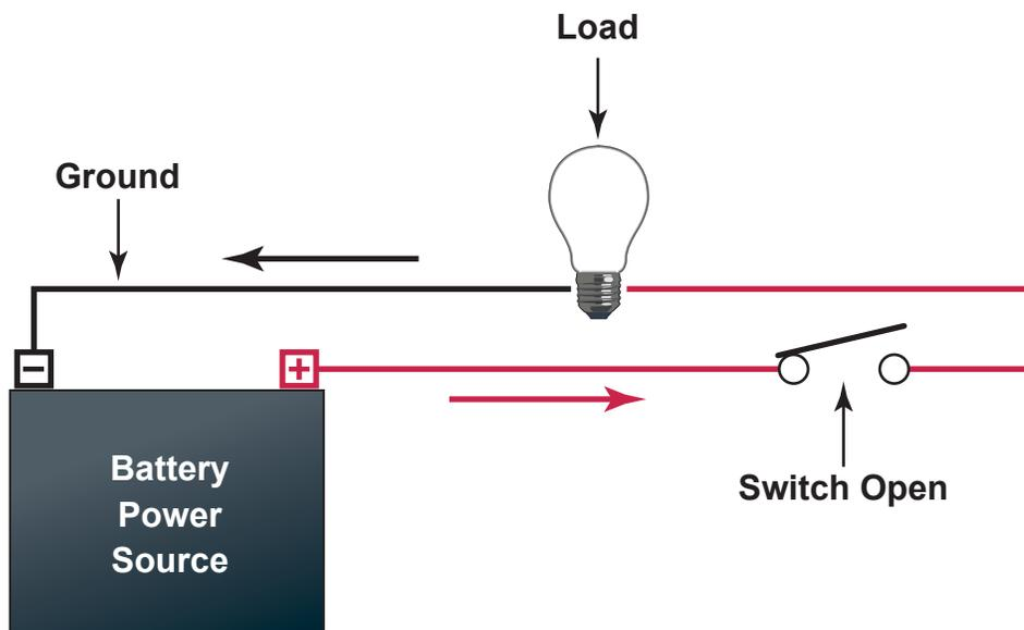
*In this electrical circuit the switch is in the open position. This circuit has been turned off. This is an “open circuit”. The switch symbol is similar to a draw bridge over a river. When the draw bridge is up, no traffic can cross the river. No power is being supplied to the load in this drawing.*
