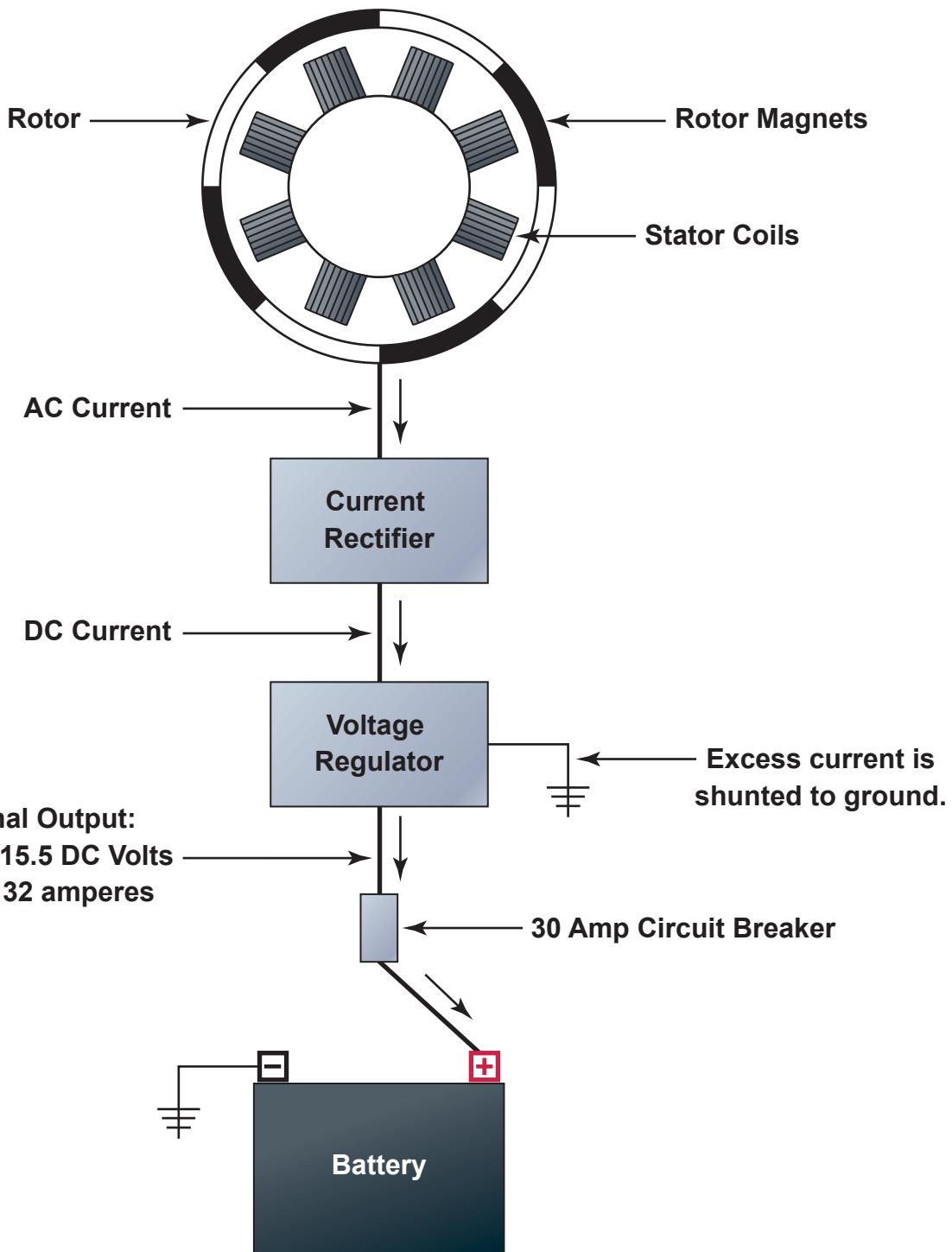
*The three-piece alternator is the most common as used on motorcycles.*
